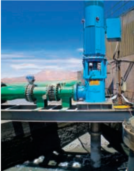
Figure 2. Vertical turbine pump—All wetted parts made of Duplex 2205 designed to handle large amounts of solids
