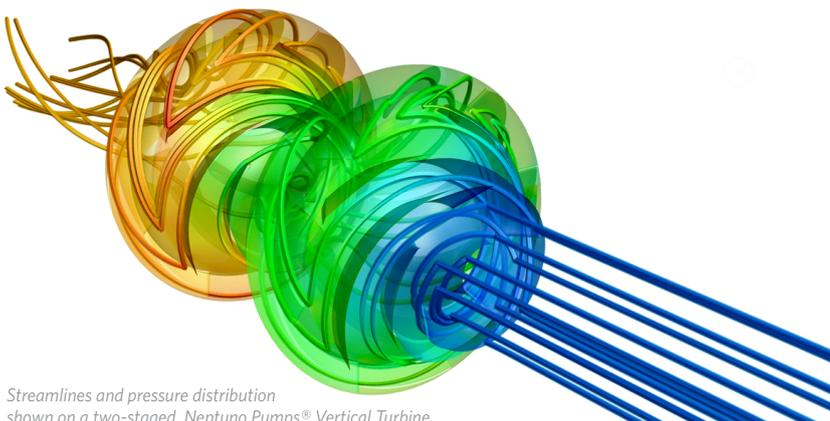
*Streamlines and pressure distribution shown on a two-staged Neptuno Pumps® Vertical Turbine.*
